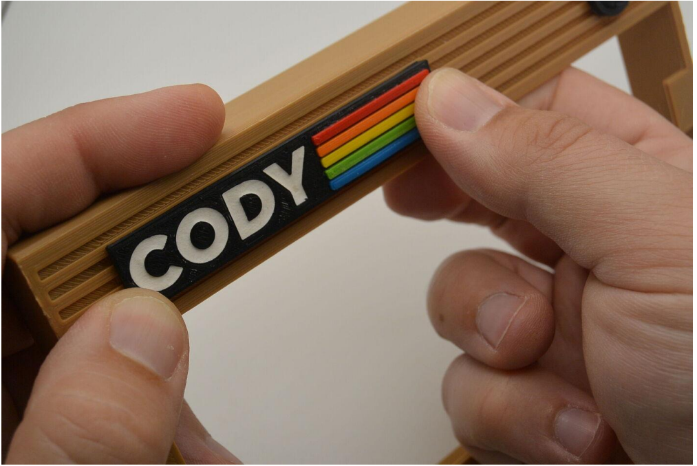
The case badge being glued into the case top. The LED holder is visible in the background.
