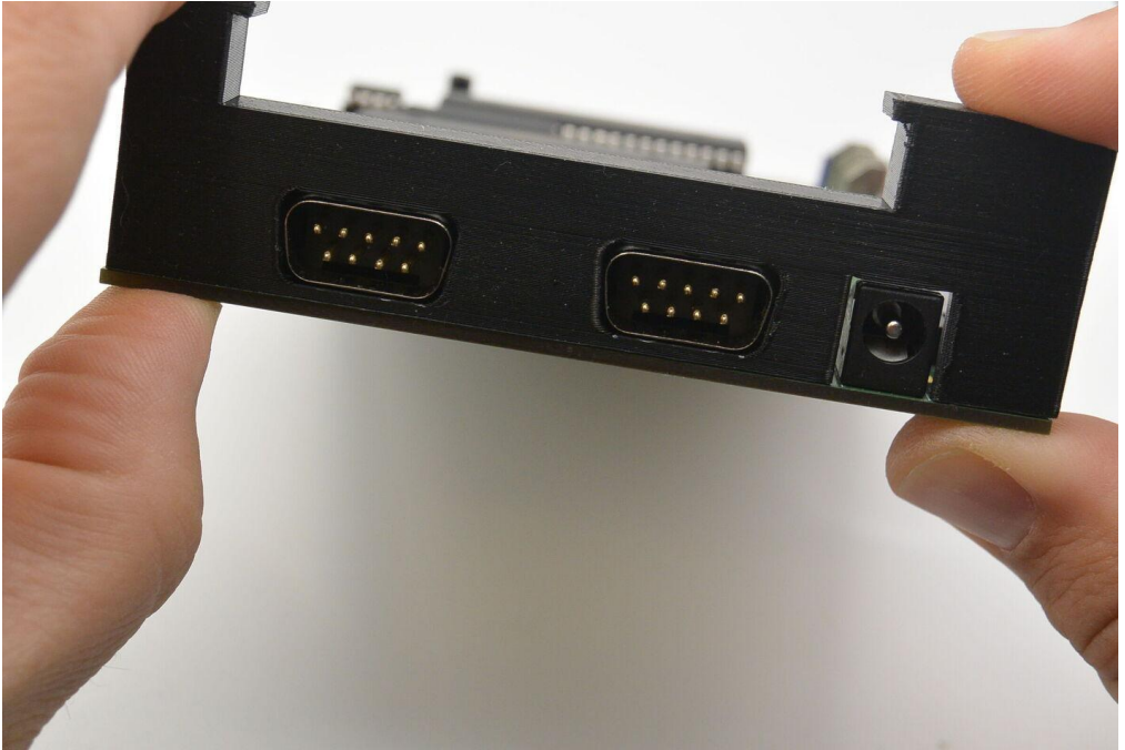
Testing the keyboard bracket's fit with the joystick and power connectors.
